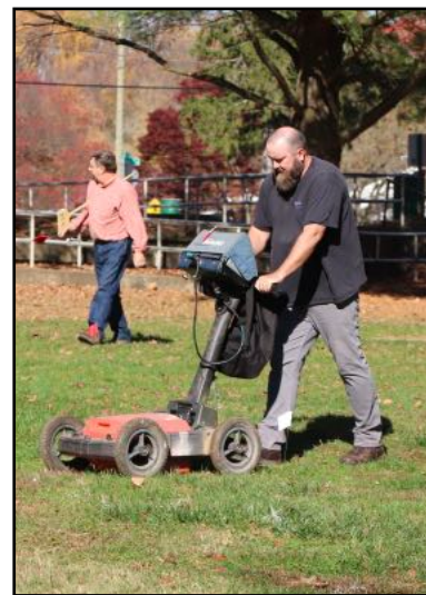
Jay Graf walking his GPR unit across the grid in search of the hotel. Photo by Angela Evans
