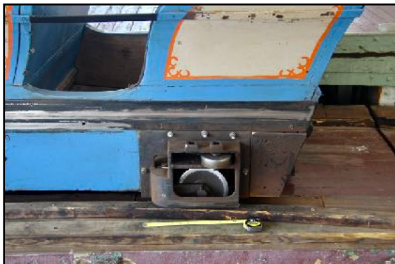
Photo of the Leap the Dips Coaster car showing the bottom and side wheels. Photo by Mark Lawlor
