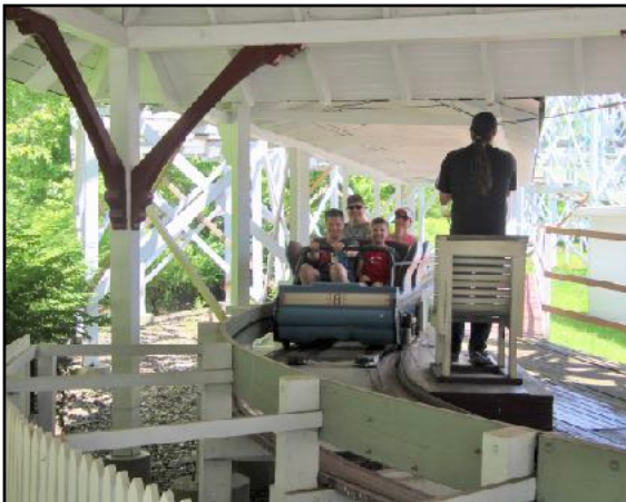
← Left Photo of the Leap the Dips Coaster at the end of the ride. Brake boards can be seen under car. Photo by Mark Lawlor
